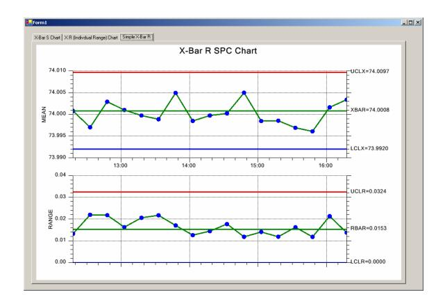
Variable Control Charts are for use with sampled quality data that can be assigned a specific numeric value, other than just 0 or 1. This might include, but is not limited to, the measurement of a critical dimension (height, length, width, radius, etc.), the weight a specific component, or the measurement of an important voltage. Common types of Variable Control Charts include X-Bar R, X-Bar Sigma, Median Range and Individual Range charts.
